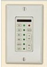
The **8270CS 6-Source Selector with IR Repeater** allows you to control volume and select components, plus feature MUTE and ON/OFF system control via an IR function. Imprinted replaceable key caps for source selections let you customize your installation. This wall controller installs in a single-gang box with a small depth.
